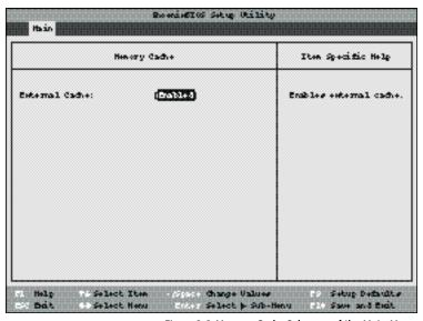
Figure 3-3 Memory Cache Submenu of the Main Menu
